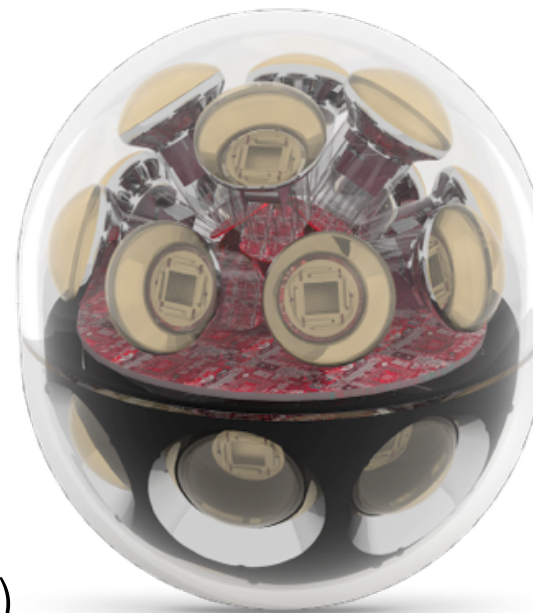
Multi-PMT DOM (mDOM) 24x3" PMTs, new glass similar to D-Egg
