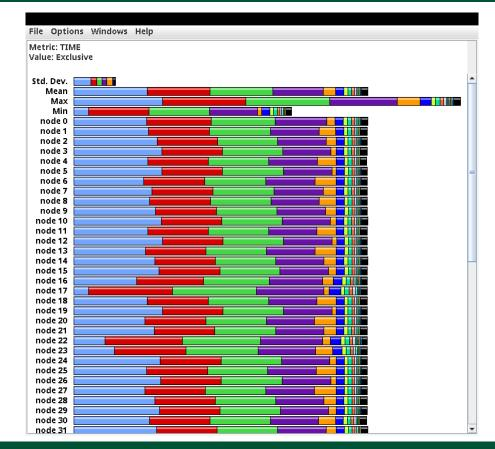
Each line is a different process/thread of execution, each color is a different function
