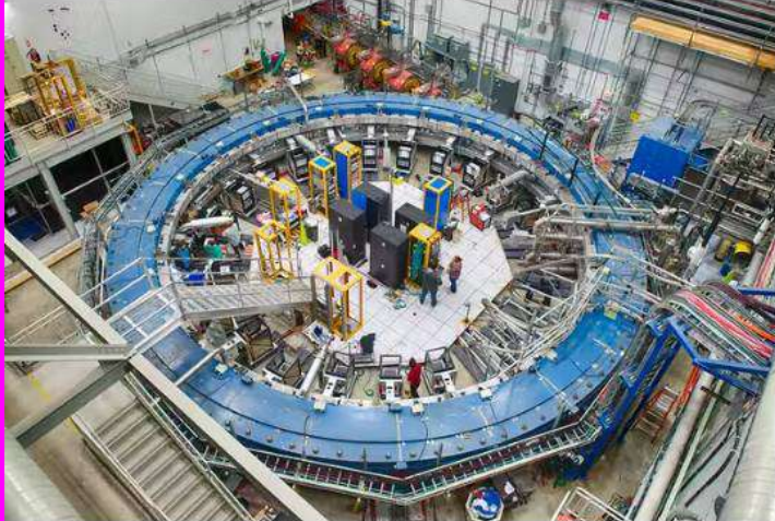
The storage-ring magnet for the Muon G-2 experiment at Fermilab. Reidar Hahn/wikipedia, CC BY-SA
