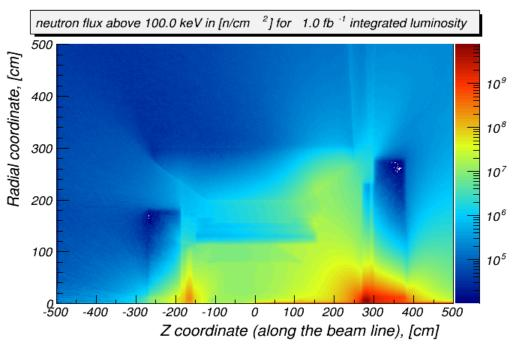
→ forward EmCal: up to ~5\*10<sup>9</sup> n/cm<sup>2</sup> per fb<sup>-1</sup> (inside the towers); perhaps ~5 less at the SiPM location
