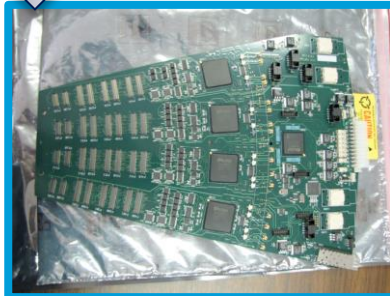
MVTX RU, 200M ch ALPIDE (ALICE/sPHENIX), FPHX (PHENIX)
