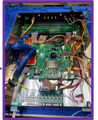
Global Timing Module (NSLS II/sPHENIX) Receiving from RHIC RF low glitter clock source
