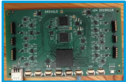
Precision timing digitizer DRS4GIO (SBIR/LDRD)
