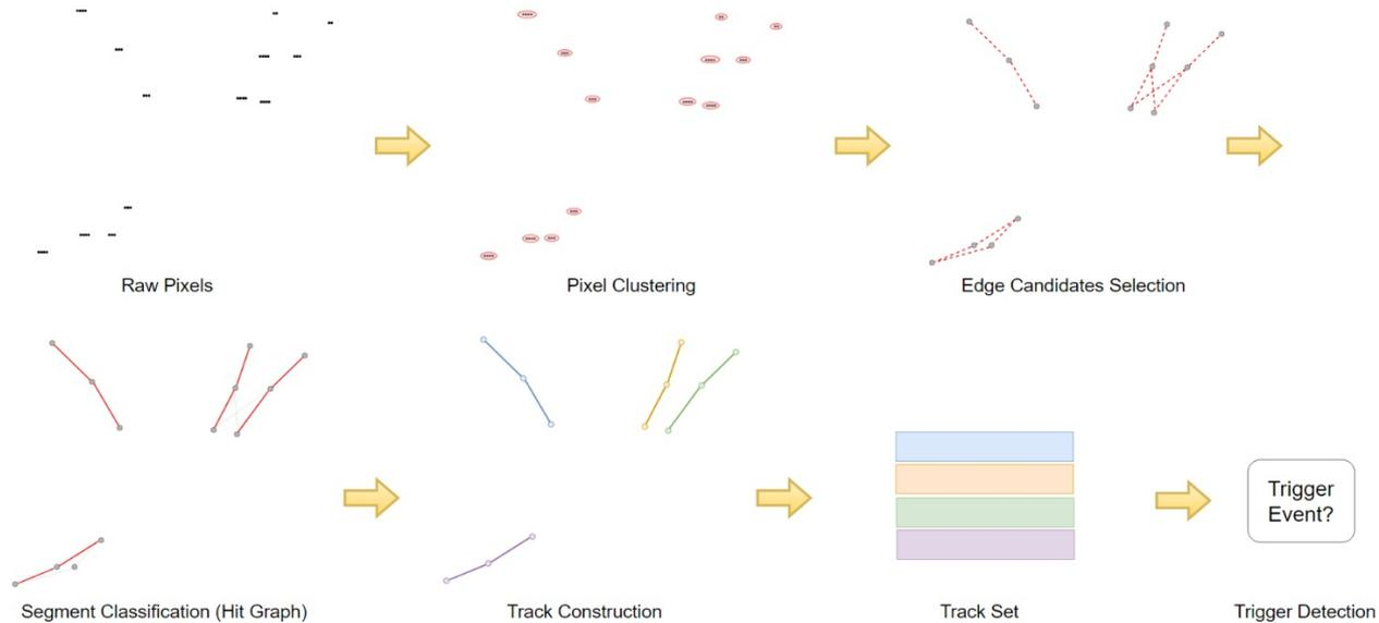
Fig. 3: Trigger Detection Pipeline with All the Steps.
