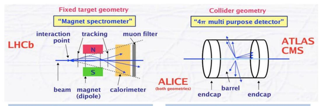
Look at collision products in a small open angle along beam axis Plane detectors perpendicular to beam
