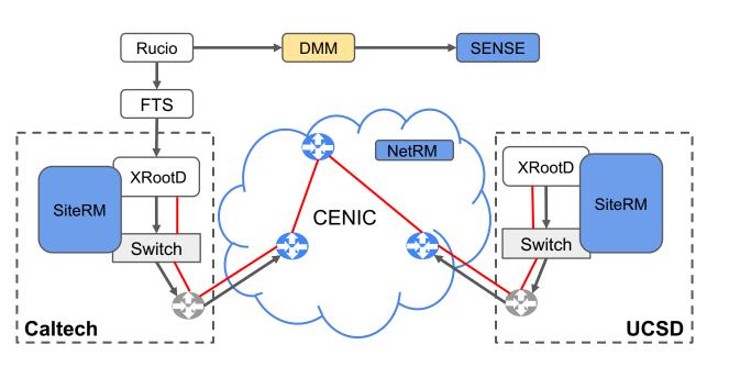
For every Rucio request, Rucio contacts DMM to ask for the IPv6 endpoints to use before contacting FTS
