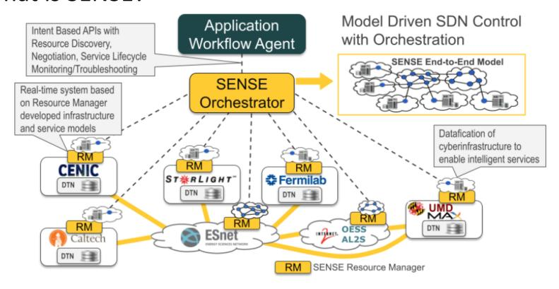
The Software-Defined Network for End-to-end Networked Science at Exascale (SENSE) system includes a model-based architecture, implementation, and deployment which enables automated end-to-end network service instantiation across administrative domains. (<a href="https://sense.es.net">https://sense.es.net</a>)
