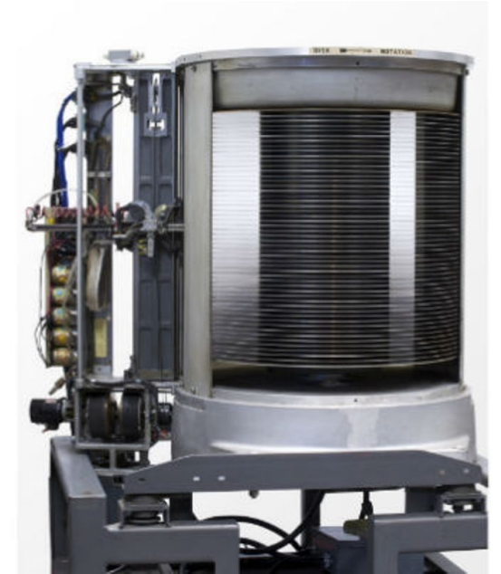
IBM 5 MB hard drive. Size of a refrigerator.
