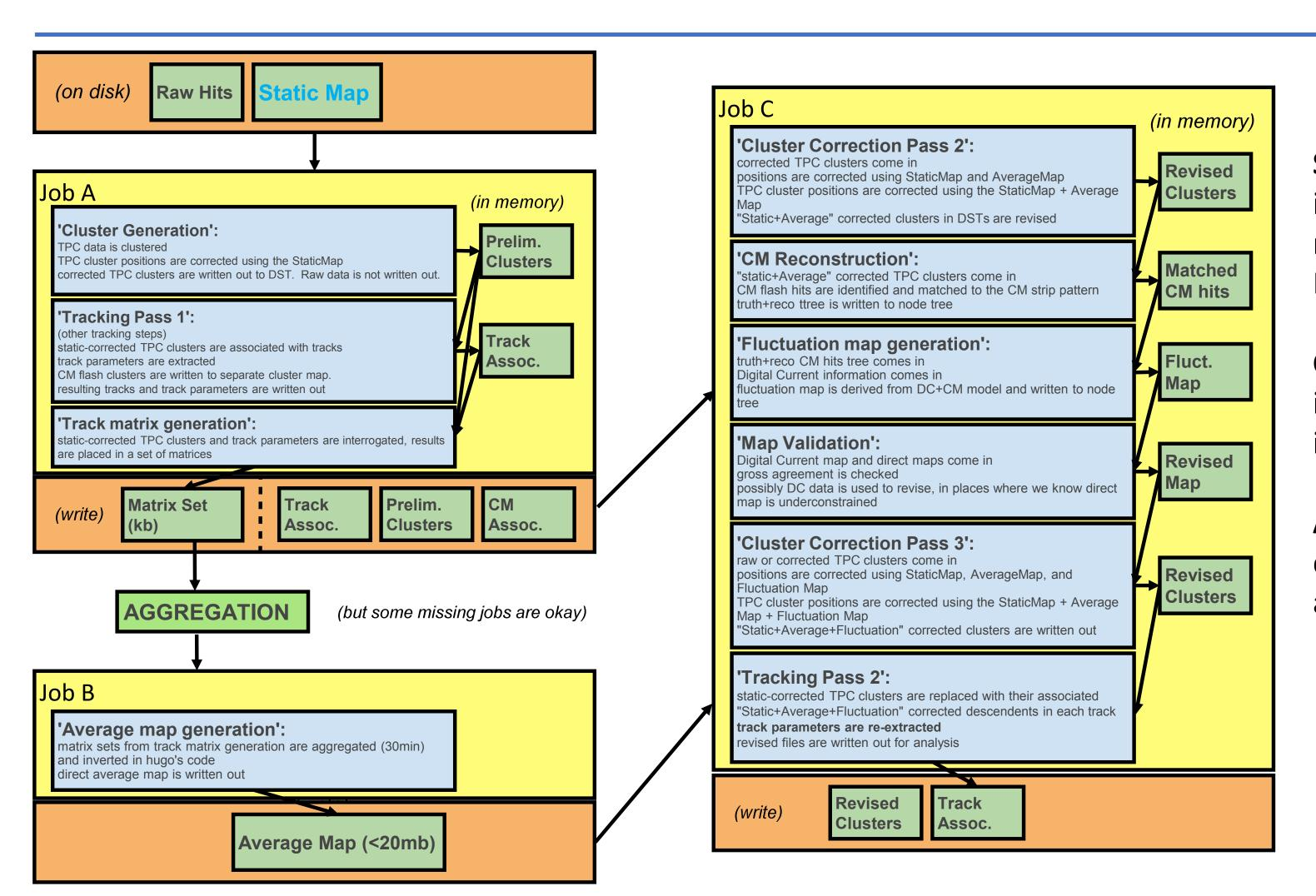
**Static Map**: Space charge independent distortions (e.g. magnetic field), created from Laser flashes without beam
