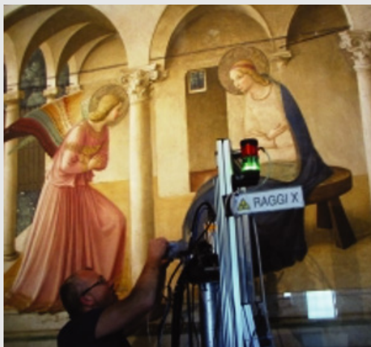
X-Ray Fluorescence (XRF) study by INFN-CHNet Firenze on "L'Annunciazione" by Beato Angelico (Museum "San Marco" - Firenze, Italy).
