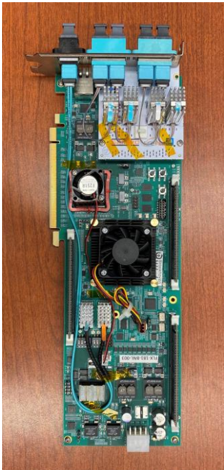
Assembled 24ch FLX-181 with 25 Gbps FireFly FMC+
