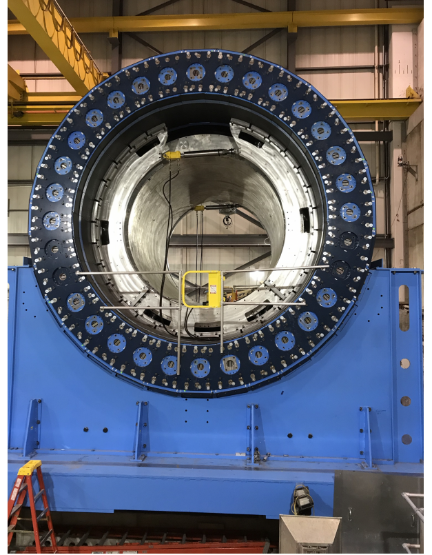
Figure 4: The BaBar solenoid in late February 2022, during installation in the sPHENIX experiment. The solenoid is surrounded by the barrel outer hadronic calorimeter and flux return. The barrel flux return (outer hadronic calorimeter) and BaBar solenoid are items planned to be reused by the ECCE experiment. The experimental cradle may also be reused.
