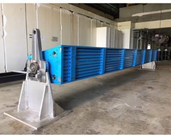
**Assembly Detail:** 5 scintillators/tower 48 towers per sector 32 sectors; 1536 channels (7680 SiPMs)
