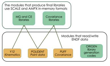
The processing codes use AMPX's in-memory structures, which are in turn populated by "wrappers" that directly access the **FNDF or GNDS** formatted files.
