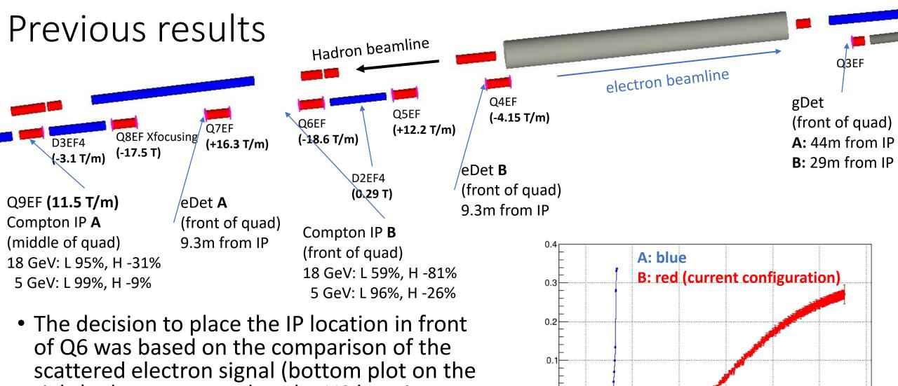
scattered electron signal (bottom plot on the right) where we saw that the US location produced a very distorted signal that was very close to the beam
