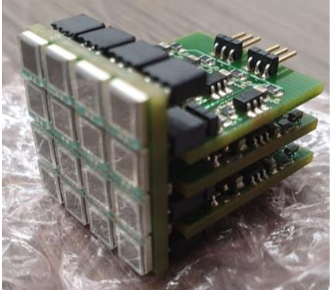
Readout module for 1 crystal with 16 SiPM
