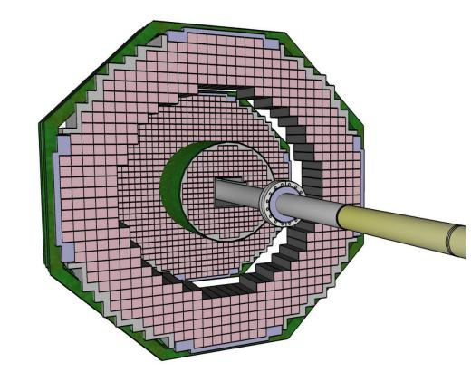
Other option being explored: addition of an inner calorimeter attached to the beampipe
