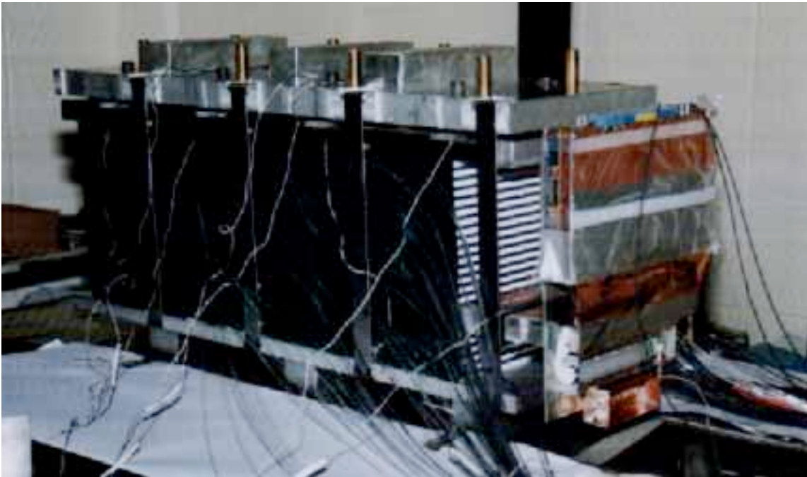
Figure II.2.3-3 Picture showing assembling of the prototype module for the test beam run 1997(compression stage).
