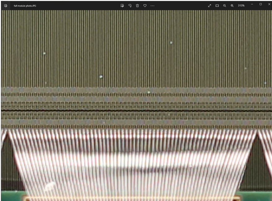
25 micron diameter aluminum wires
