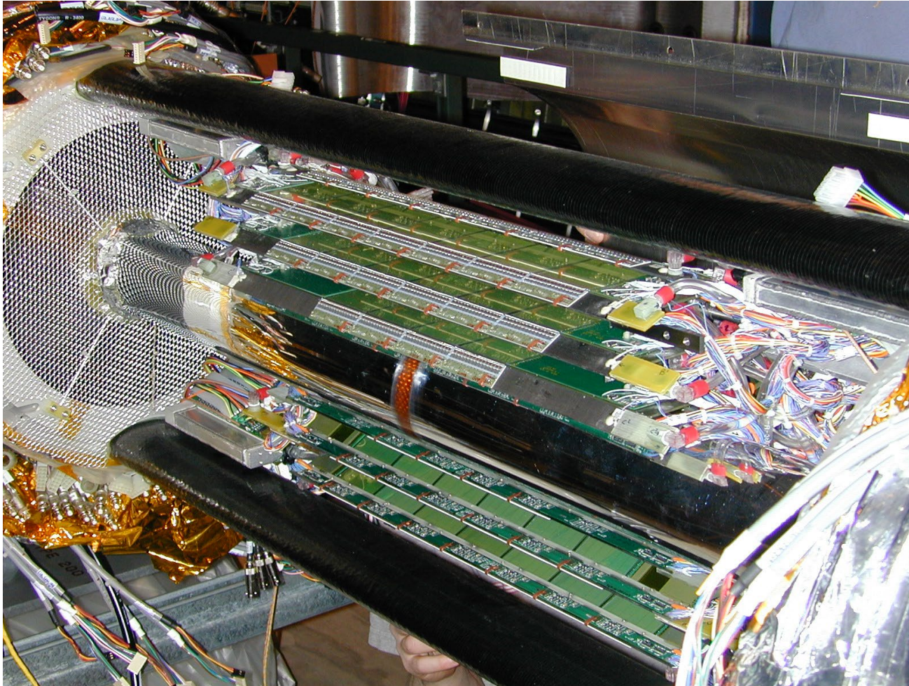
Half of Silicon Vertex Tracker Installed at RHIC
