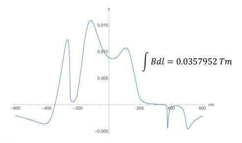
We Need shielding of the RCS beam pipe to bring fields down by a factor of 5 to bring cumulative loss < 1%
