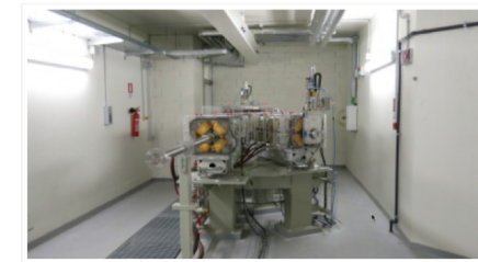
The two beamlines in the Trento Protontherapy Centre research room.
