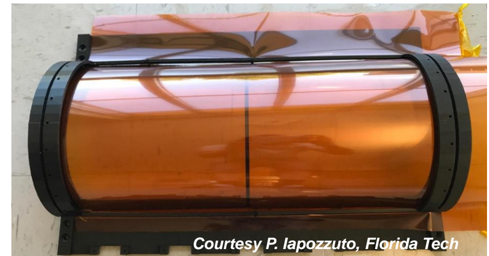
Cylindrical \mu RWELL: mechanical mockup
