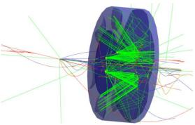
sPHENIX TPC streaming data frame, also presented in 3D zero-suppressed sparse matrix (R-phi-time) marked with signal/background hits
