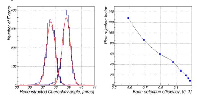
• Left: reconstructed Cherenkov angle peaks for a 50:50 mix of 50 GeV/c kaon and pion tracks at  $\eta$  = 2.4 are ~3 $\sigma$  apart (C2F6 radiator). Right: dependency of pion rejection factor on kaon detection efficiency with the selection cu varying between 37.6 mrad and 38.4 mrad applied to the left hand side plot.
