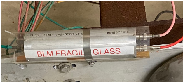
Beam Loss Monitor
