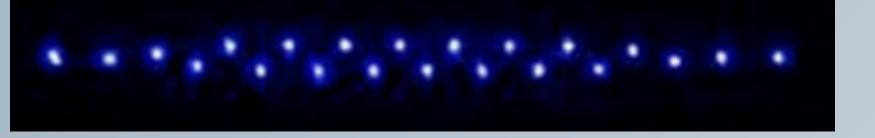
The model of a one-dimensional ion coulomb crystal basically uses the coupled harmonic oscillators with the coulomb interaction acting as the spring constant between the masses.
