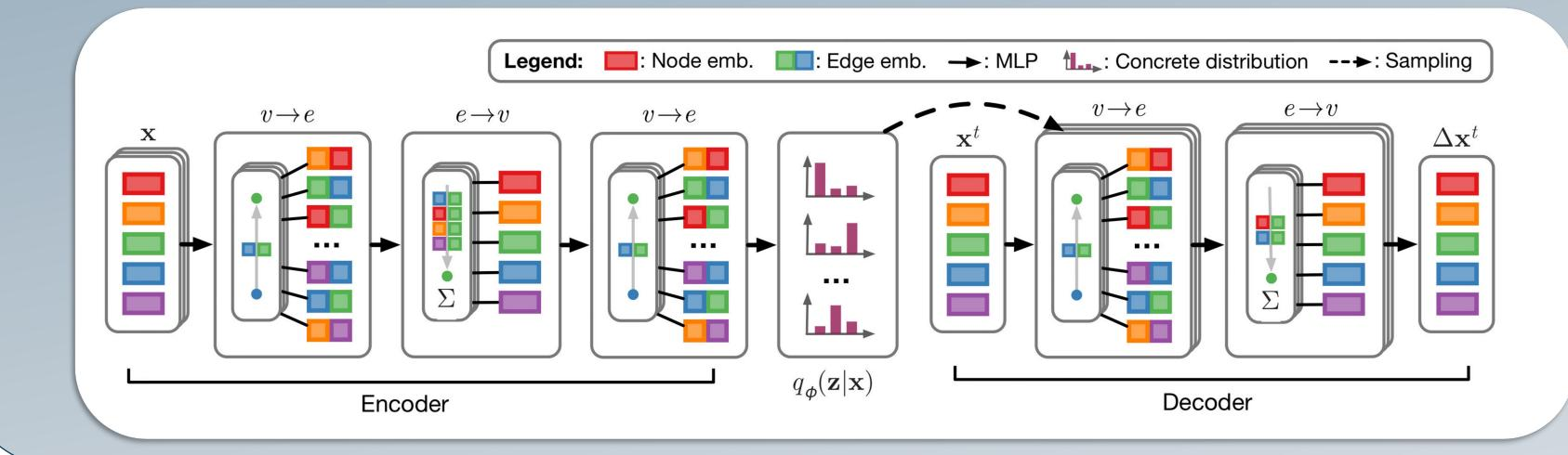
The NRI model learns the dynamics with a Graph NN over a discrete latent graph and performs inference over these latent variables. Jointly trained an encoder that predicts the interactions given the trajectories, and a decoder that learns the dynamical model given the interaction graph. **Discuss:** For the particle motion prediction, the forces diverge when the distance between particles goes to zero, It can cause issues when integrating with fixed step size.
