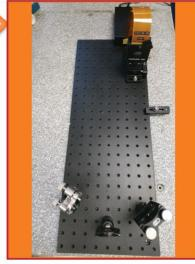
Shaping optics are usually placed close to the photocathode, and diagnostic elements are also as close to the photo-emission gun as possible to provide accurate measurements of laser parameters on the photocathode.
