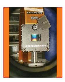
This will also enable the use of a spatial light modulator (SLM) between the two harmonic generation crystals for intensity control of the second harmonic of the ATF Nd:YAG laser at 532 nm. Subsequent fourth harmonic generation and image relaying will allow the profile at the photocathode to be controlled and optimized.
