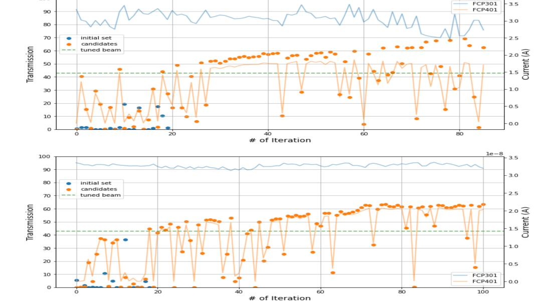
Best initial tune by operator ~ 40 % beam transmission Best achieved by ML model ~ 70 % beam transmission
