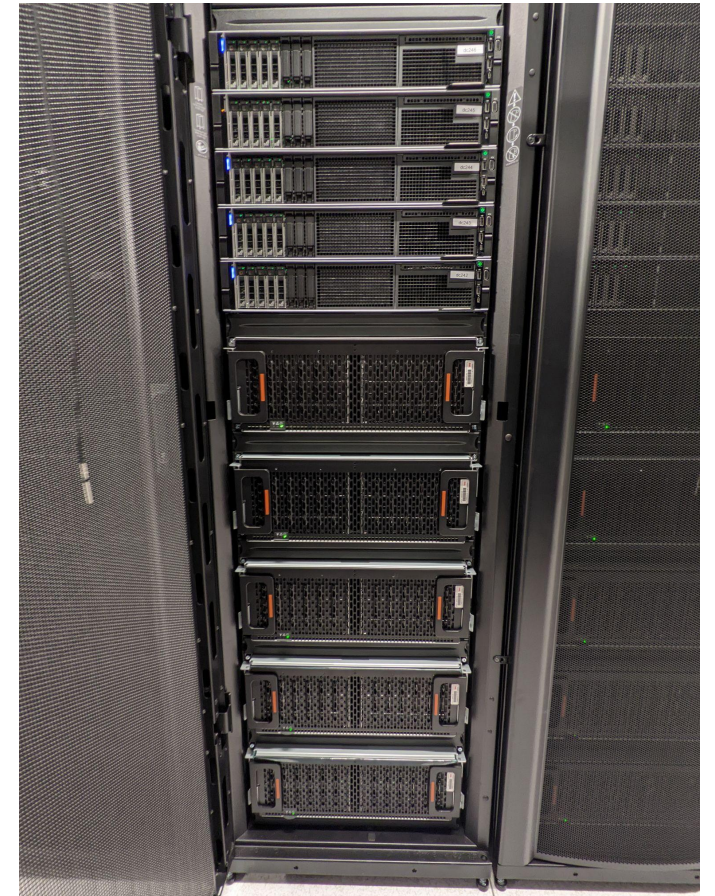
Western Digital Ultrastar Data 102-bay JBODs with Dell R740 headnodes
