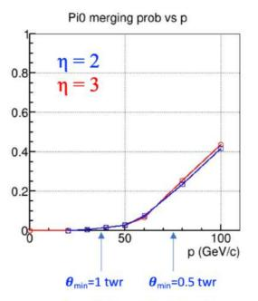
Can effectively discriminate  $\gamma/\pi 0$  even when two photons are separated by 0.5 tower size
