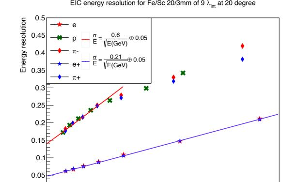
Hypothetical variant, 9 interaction lengths long calorimeters. Same structure for Ecal and Hcal sections. Three different technologies:
