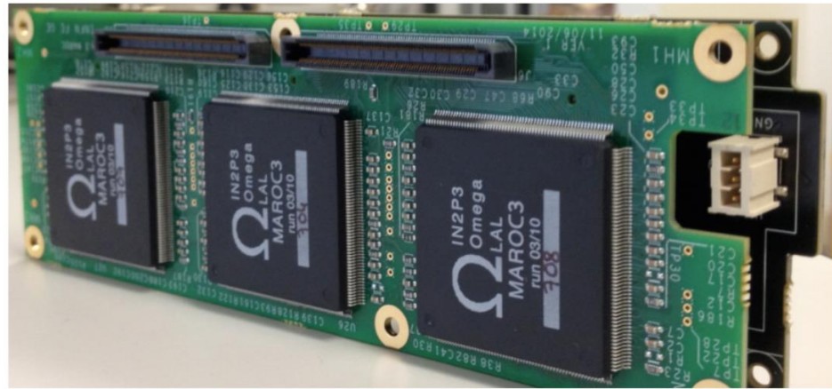
ASIC board produced for the RICH detector for CLAS12 with MAROC chips installed
