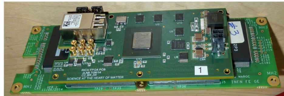
FPGA Board Screenshot for the RICH detector for CLAS12 with ASIC board attached
