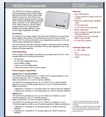
The intent is to provide batteries that meet / exceed code, which is 24h standby followed by 15m of alarm
