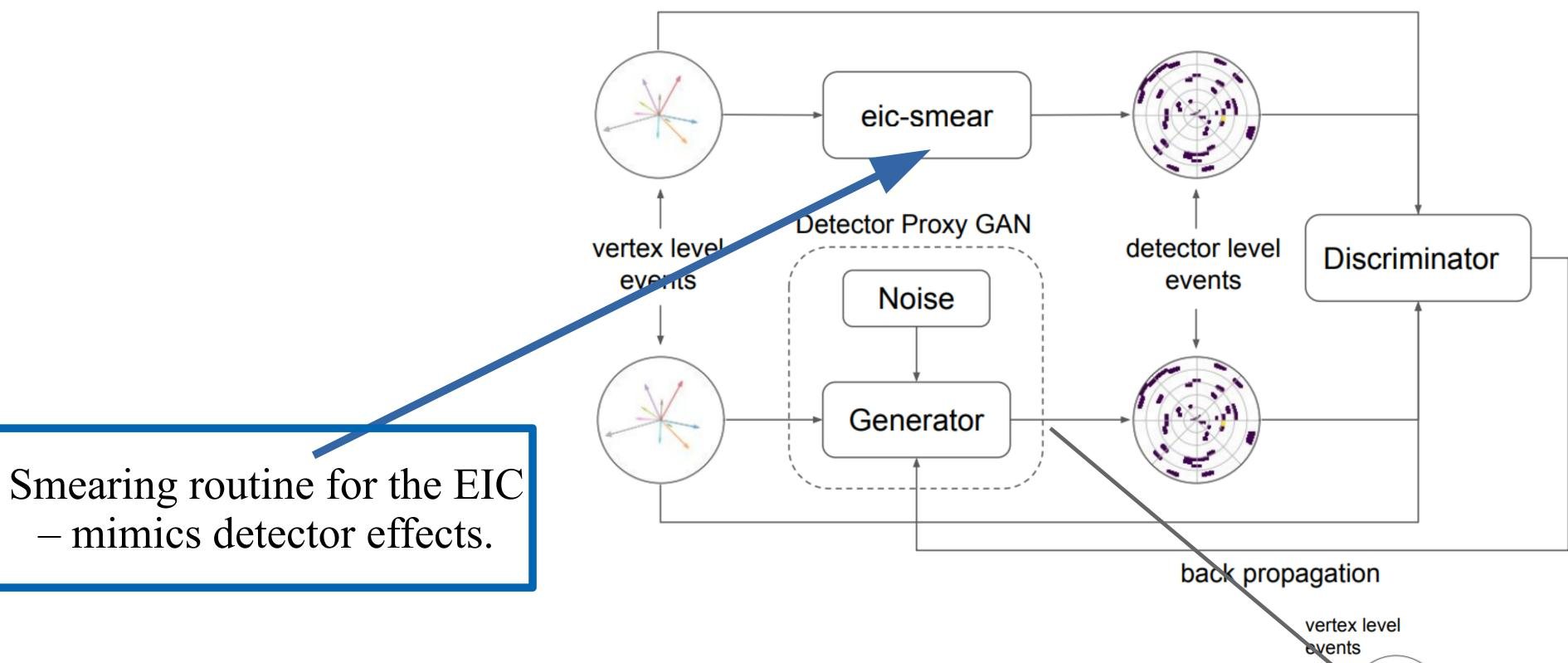
The detector proxy GAN is trained to act as simulator transforming vertex into detector events.
