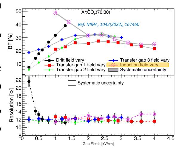
Larger induction gap field more IBF suppression due to bending to field lines at bottom of last GEM away from the holes
