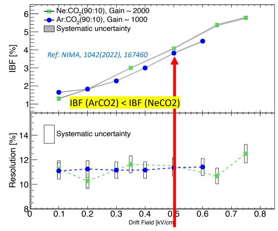
$v_{ion}$  for Ne ~ 3 x  $v_{ion}$  for Ar  $\rho(Ar:CO_2-90:10) = 2 X <math>\rho(Ne:CO_2-90:10)$ Neon based gas mixtures preferred for TPC
