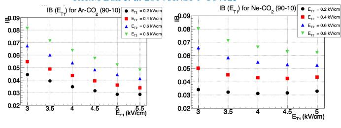
Ne-CO2 (90:10) IBF > ArCO2 (90:10) from triple GEM detector at lowest IBF configuration
