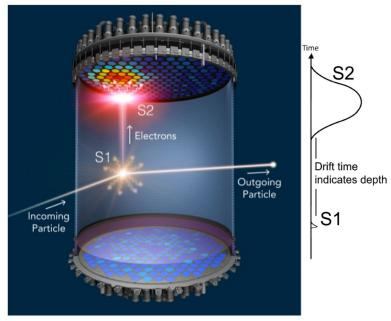
The LUX-ZEPLIN (LZ) Experiment is a direct detection dark matter experiment.
