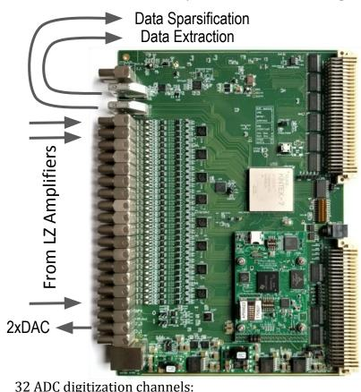
Offloading 16 custom HDMI serial links:
