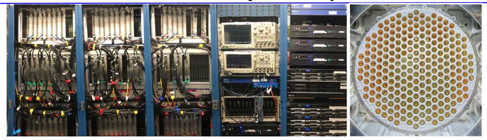
The LZ data acquisition and sparsification system (DAQ) is responsible for real-time zero suppression and event selection.
