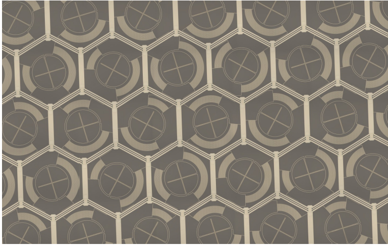
Top left: picture of a 63-pixel photometer array for SPT-3G+. The quality factor is \sim 4.8e5 .
