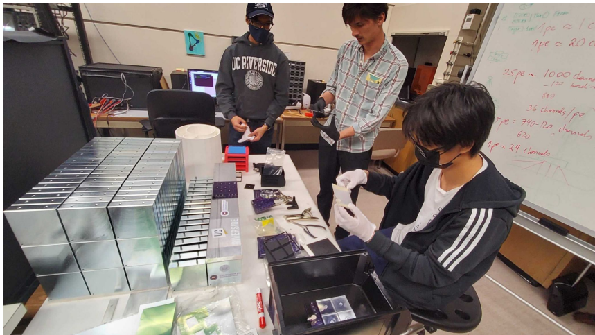
Students completing first layer of calorimeter insert prototype
