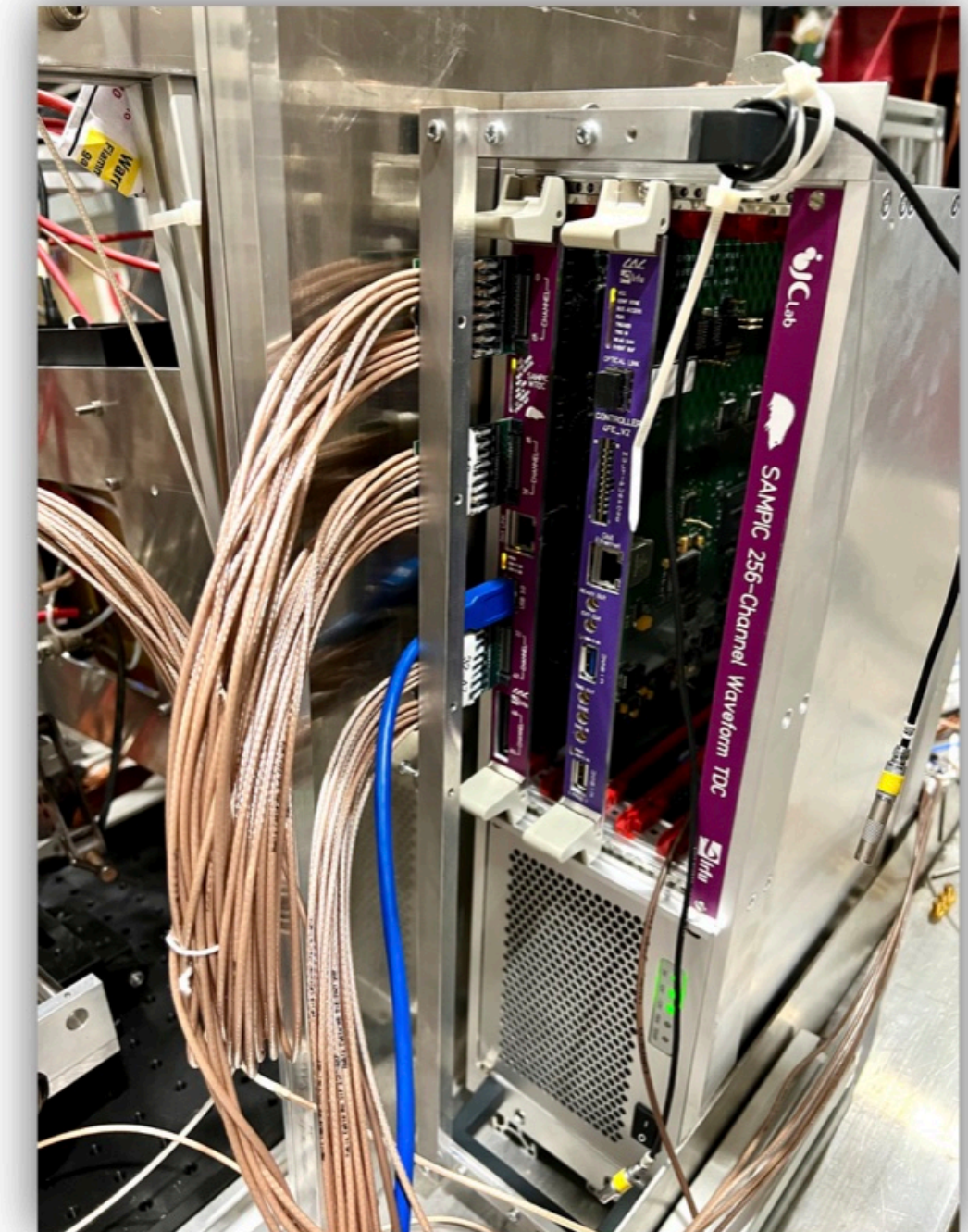
64 channel SAMPIC digitiser, J. Maalmi, D. Breton et al., CEA Saclay
