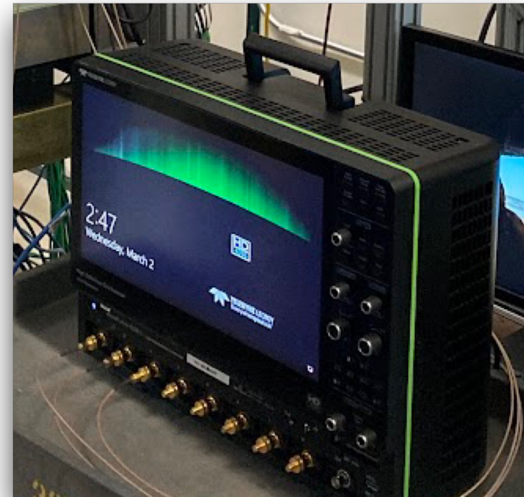
8-channel oscilloscope, 2 GHz, 10 GSa/s Large memory: take 20k events during 4 s spill
