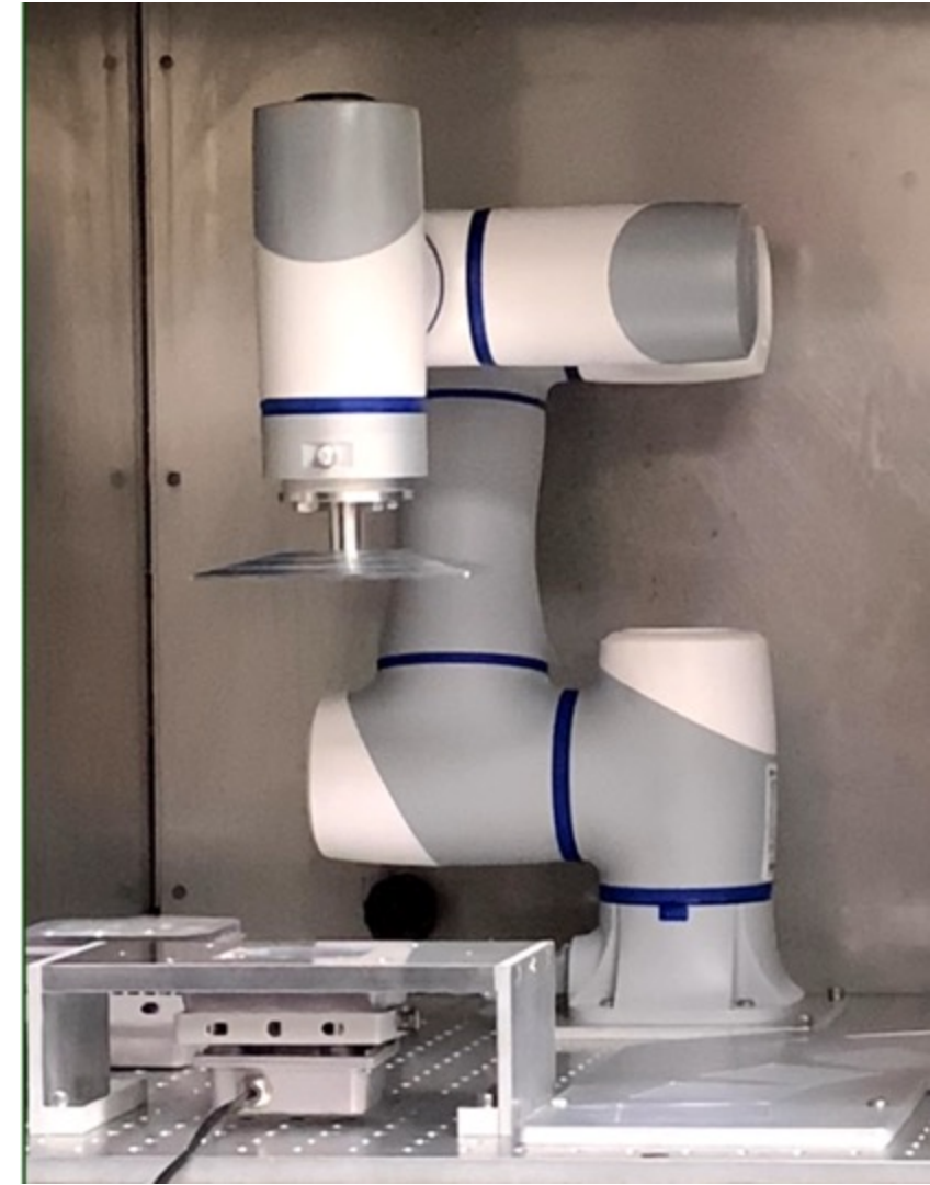
Prototype 6-axis 3D printer for scintillators
