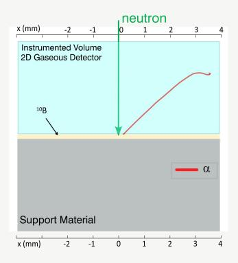
State of the Art (SoA) neutron **Position Sensitive** gaseous detectors employ a **thick layer of a material with** <sup>10</sup>**B atoms** for neutron conversion.
