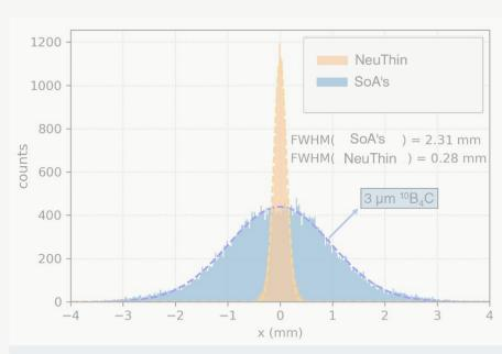
Simulations indicate the potential for position resolution improvement by a factor of ~8.
