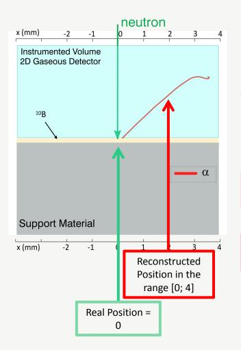
State of the Art (SoA) neutron **Position Sensitive** gaseous detectors employ a **thick layer of a material with** <sup>10</sup>**B atoms** for neutron conversion.
