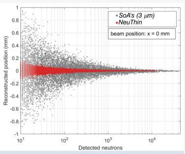
NeuThin converges to the "true position" for lower number of detected neutrons, opening the door to a reduction in the exposure time.
