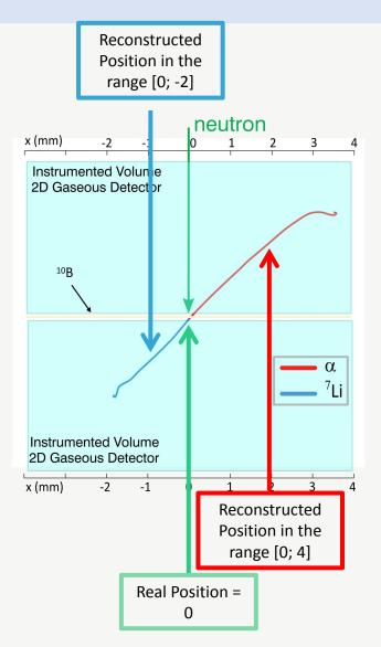
Two position sensitive gaseous detectors, instrumenting both sides of the converter foil, are required.
