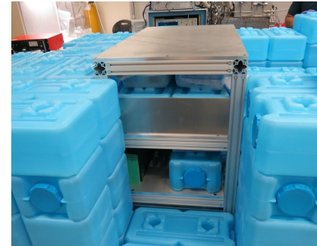
DT stand frame, constructed and partially shielded
