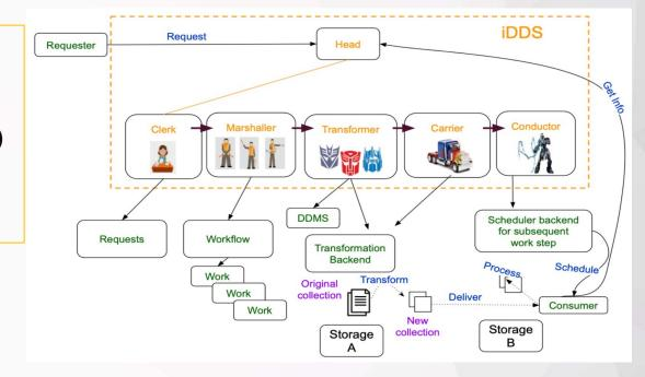
A RESTful interface processes requests to run fine grained workflows orchestrating the marshalling/transformation/delivery of data and managing multi-step processing, with complex workflow support: DAGs, subdivided workflows, loops, dynamic conditions, and so on.
