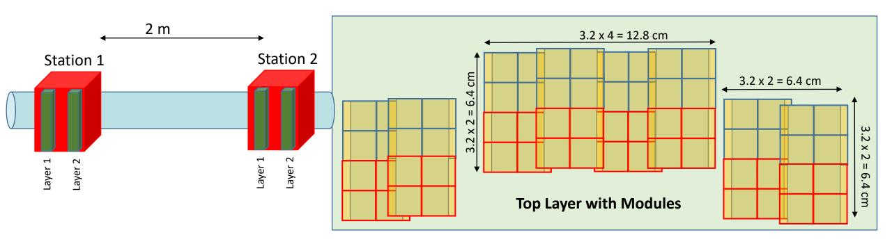
128 ASIC per layer, a total of 512 ASIC (most probably 1024 pixels per ASIC)
