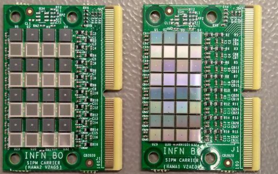
8x4 matrices with commercial Hamamatsu
