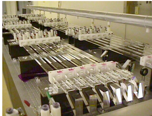
BaBar DIRC radiator bars in SLAC
