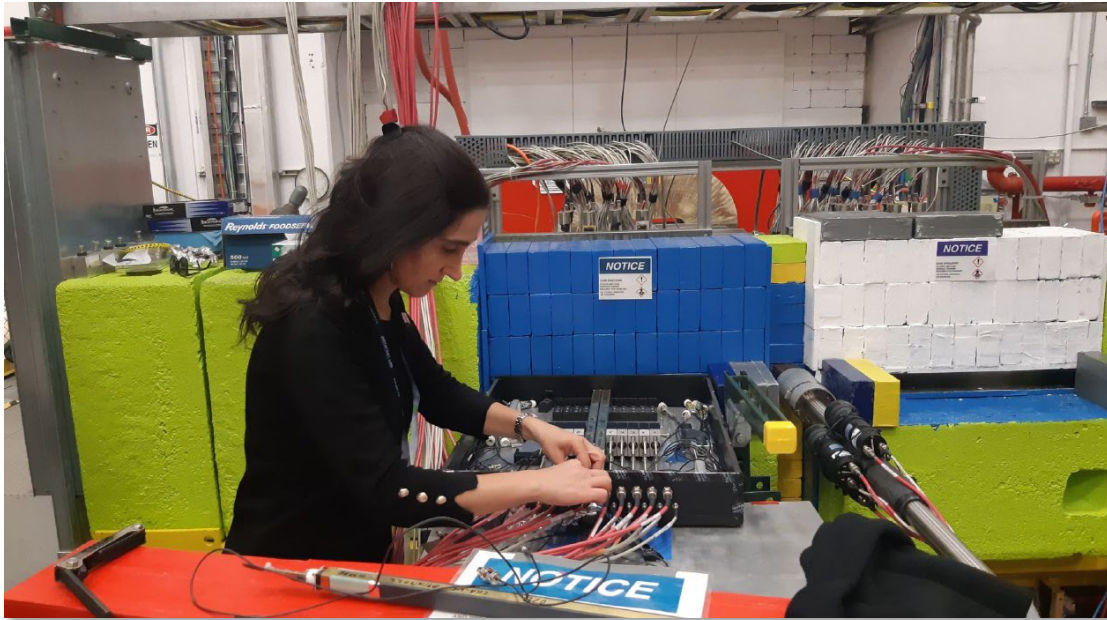
Installation of the 3x3 (40cm SciGlass) prototype in the beamline at Jefferson Lab
