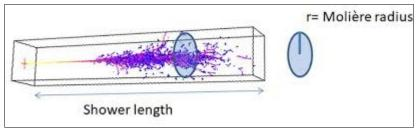
Molière radius is the radius of a cylinder containing on average 90% of the EM shower's energy deposition. For PbWO $_{4}$  it is around 2 cm.
