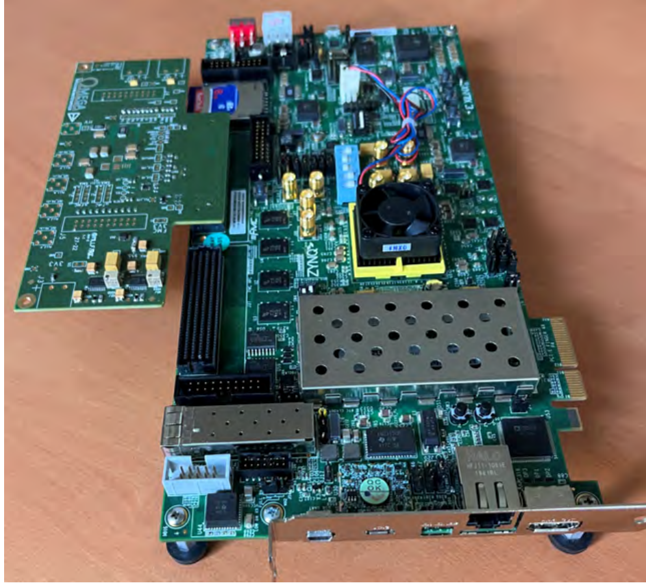
Figure 17: Picture of a bare printed circuit board connected trough FMC connector to a Xilinx ZC706.
